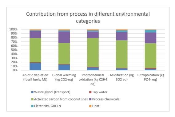
Figure 3 The distribution of the process resources in the impact categories; abiotic depletion photochemical oxidation acidification and eutrophication
