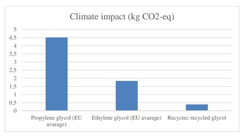
Figure 5 Comparing climate impact of virgin glycols and Recyctec recycled glycol.
